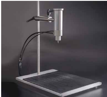
Basic stand – the test head can be combined with a sharp or blunt needle or a tube adaptor
