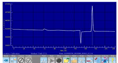
The BevAlert Total Sulfur GC detects parts-per-billion levels of total sulfur in beverage-grade carbon dioxide. A fixed volume of sample is injected and passes through a compact, high-temperature reduction reactor where undesirable sulfur-containing compounds are reduced to hydrogen sulfide. Hydrogen sulfide is separated from potentially interfering components on the analytical column and elutes to the photoionization detector (PID).
