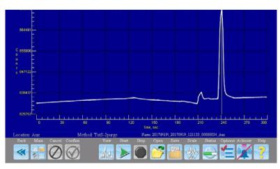
As hydrogen-based fuel cells become more widely adopted throughout various industries, ensuring sulfur-free hydrogen is a must to avoid poisoning the catalyst. The MOCON® BASELINE® 9100 (utilizing an HS-PID) can detect very low-level total sulfurs by converting all sulfurs to hydrogen sulfide using a reduction reactor.
