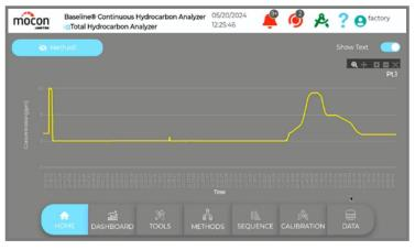
MOCON BASELINE CHA Total Hydrocarbon Analyzers are best-in-class analyzers that have been providing solutions for decades to quickly detect low-level impurities in Calibration Gases, and Food and Beverage Gases. The latest version of CHA Analyzers includes a graphing function that allows the user to easily see any excursions or trends in the data. Alarms can be set to inform users if and when impurities are too high for an application, allowing for immediate corrections.
