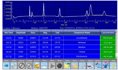
The BevAlert<sup>®</sup> Gas Chromatograph (GC) can be applicated to detect acetaldehyde, methanol, benzene, toluene, ethylbenzene and xylenes well below the recommended International Society of Beverage Technologists (ISBT) detection limits. For this application, the GC will utilize a dual-column configuration. The pre-cut column will remove interfering heavier components and moisture, reducing analysis time and protecting the analytical column.
